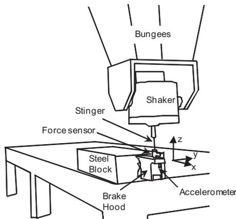
Fig. 4. Experimental setup for measurement of brake hood dynamic response
