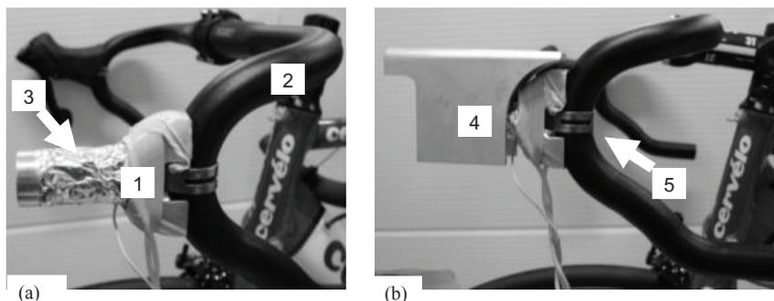
Fig. 1. Photographs of the brake hood force transducer. (a) Instrumented body mounted on handlebar and (b) hand rest covering the instrumented body (1- Transducer instrumented body, 2- Handlebar, 3- Aluminium foil covering strain gauges, 4- Hand rest, 5- Fixing clamp)
