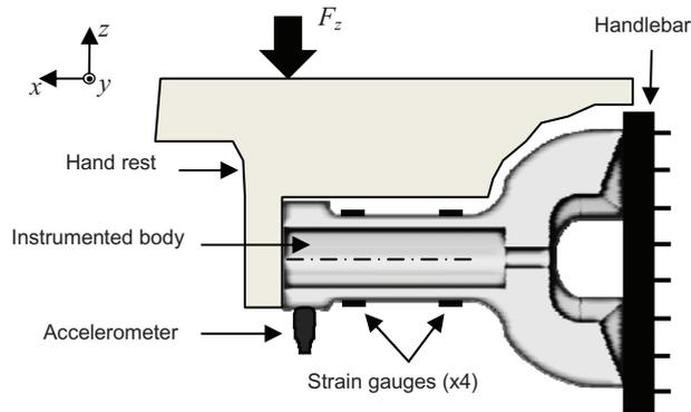
Fig. 2. Sectional view of brake hood force transducer. Strain gauges locations are indicated
