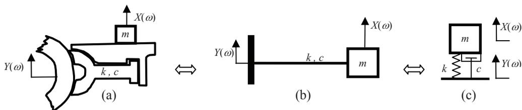
Fig. 3. Model of brake hood base excitation problem ((a) brake hood fitted to handlebar; (b) one DOF cantilever beam model; (c) spring-mass-damper system equivalent to (b))
