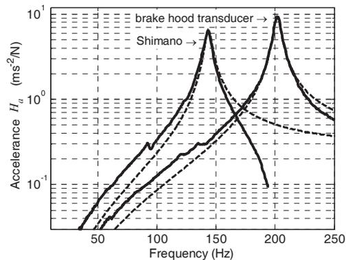
Fig. 5. Accelerance of Shimano brake hood and brake hood force transducer (----- model; ————— experimental measurements)
