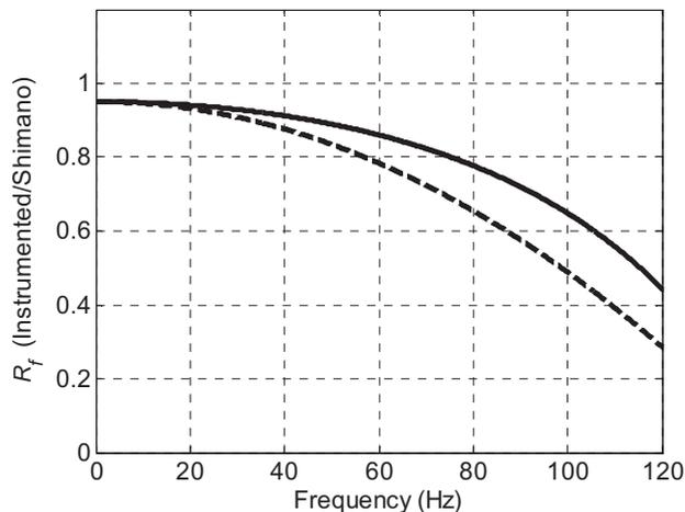
Fig. 6. Force ratio  $R_f$  between measured force by the BHFT and the standard brake hood (— actual BHFT; - - - - stiffer BHFT)
